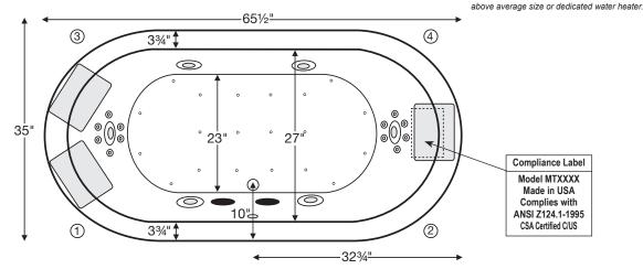
Numbered areas outside of tub represent possible stub-out locations for cleaning systems and Breda valves.
